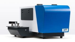
The Nexis GM is designed to connect pressurized Gas of LPG sample cylinder easily and safely in order to safely load the sample loop connected to the 10-port valve of the NEXIS GM, where a fixed volume of sample will be introduced to the TSHR 6000 and 7000 series TN/TS/TX Analyzer. The NEXIS GM is standard equipped with two sample loops: one sample loop with a volume of 10 mL for gasses and one sample loop with a volume of 100 uL for liquefied gas (LPG) samples.
